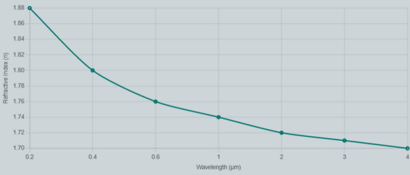
Sapphire ( $\text{Al}_2\text{O}_3$ ) provides broad optical transmission from 0.20  $\mu\text{m}$  to 5.5  $\mu\text{m}$ , covering the UV, visible, and mid-infrared regions. With its higher refractive index (~1.76) and excellent optical stability, sapphire is well suited for UV–VIS–IR imaging, laser systems, aerospace and defence optics, thermal sensors, and rugged broadband optical components.
