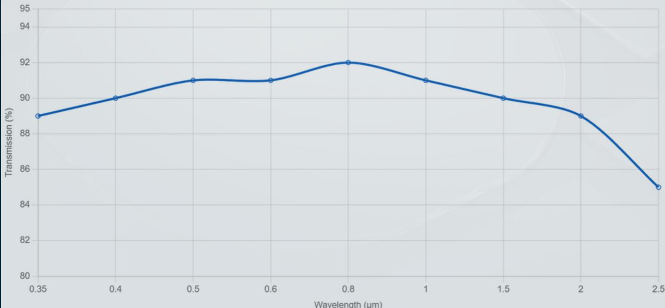
Typical transmission 350 nm – 2.5 μm, based on 1 mm sample.
