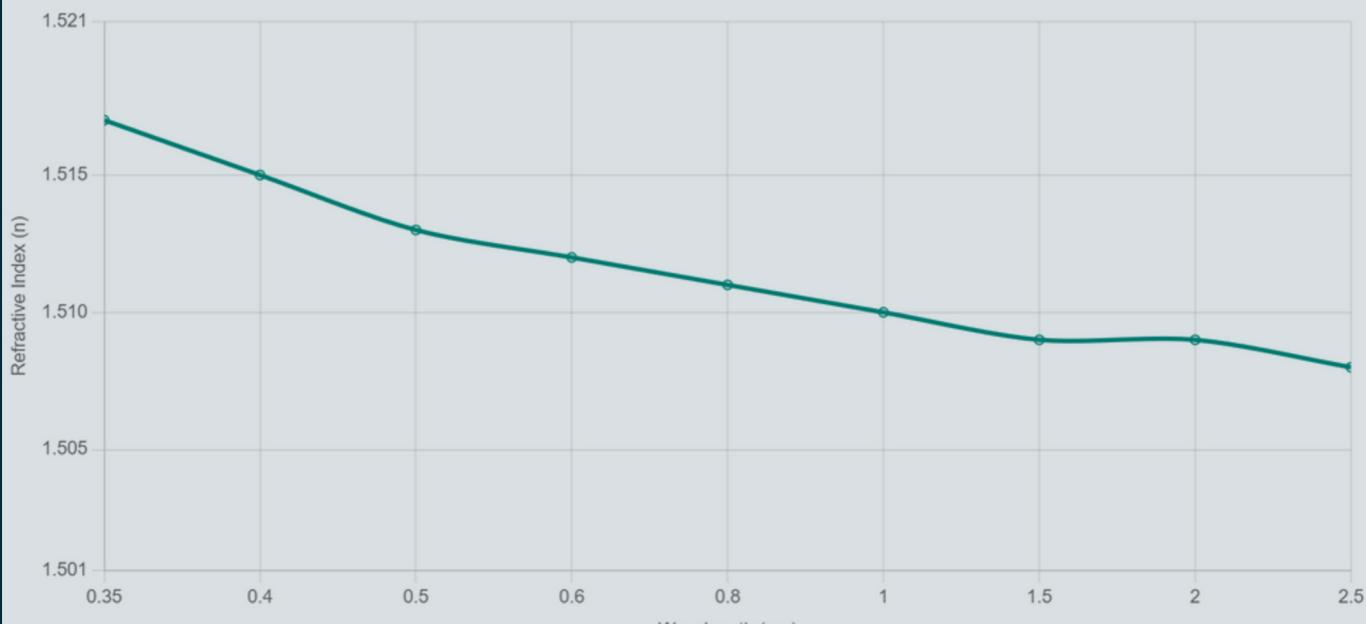
Refractive index ~1.51 @ 589 nm — minimal dispersion in visible range.
