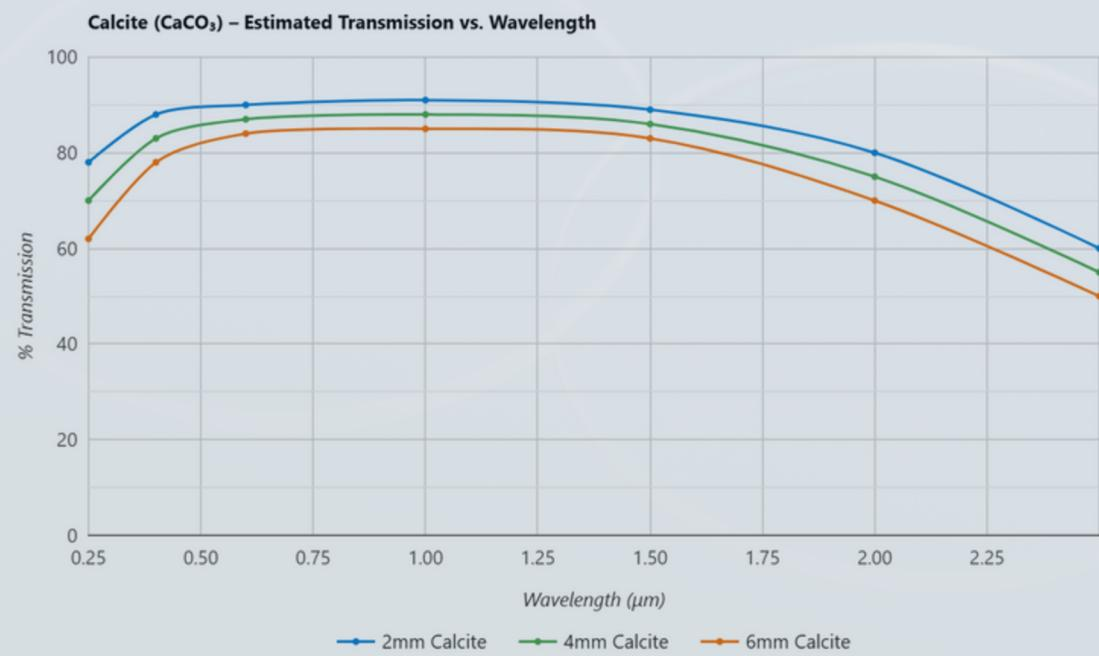
Estimated optical transmission range: 0.25–2.5  $\mu\text{m}$ , with excellent clarity in the visible region.
