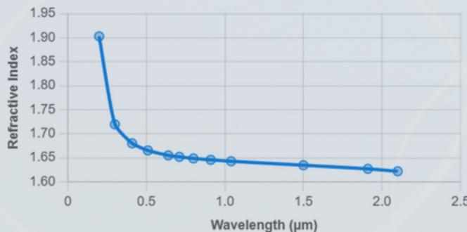
Experimental refractive index data across 0.2–2.1 μm wavelength range
